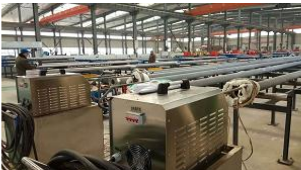
Pipe flange weld joint heat treatment
