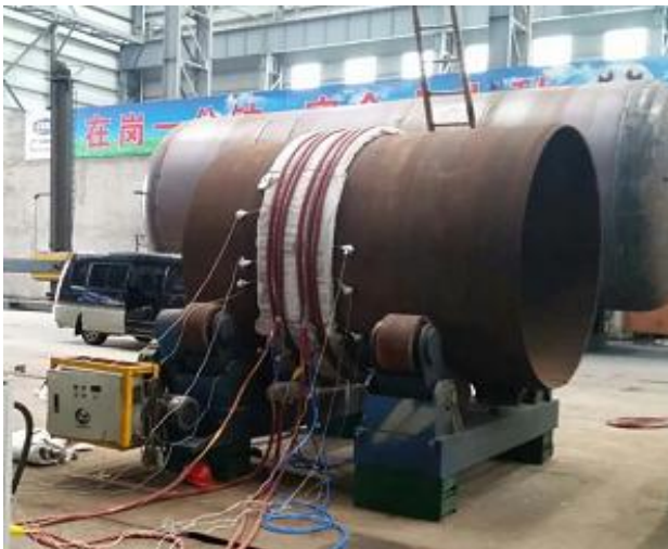
Pipe flange weld joint heat treatment
