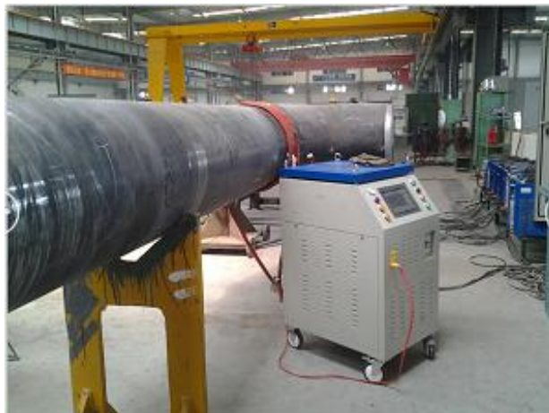
Pipeline weld heating
