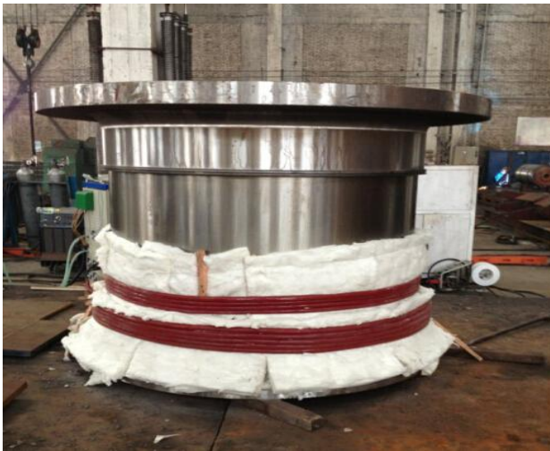
Press vessel weld preheat and PWHT
