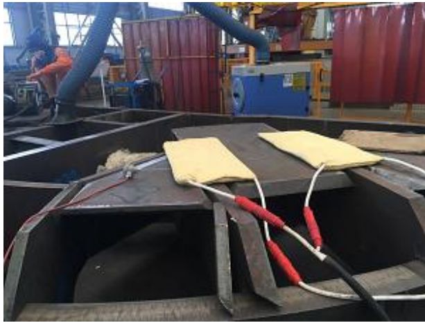
Pipeline heating before welding
